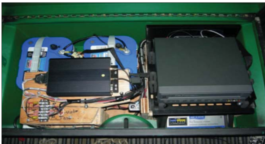
Bait car hardware fitted inside reinforced box of a utility.
