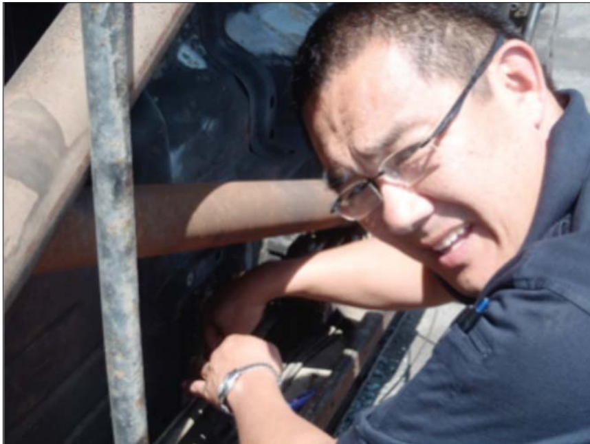
Lifting a secondary VIN from chassis rail of an impounded vehicle
