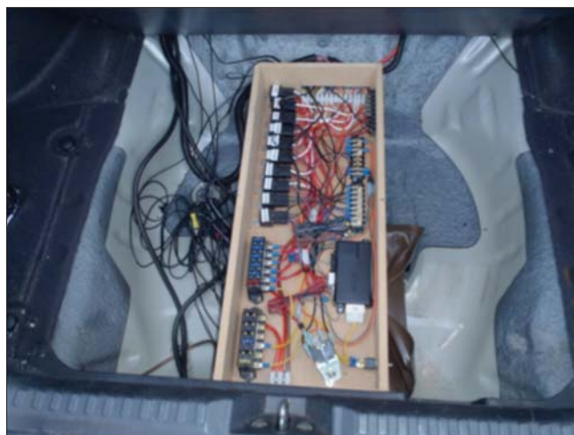
Spare tyre well to house wiring and equipment for bait car
